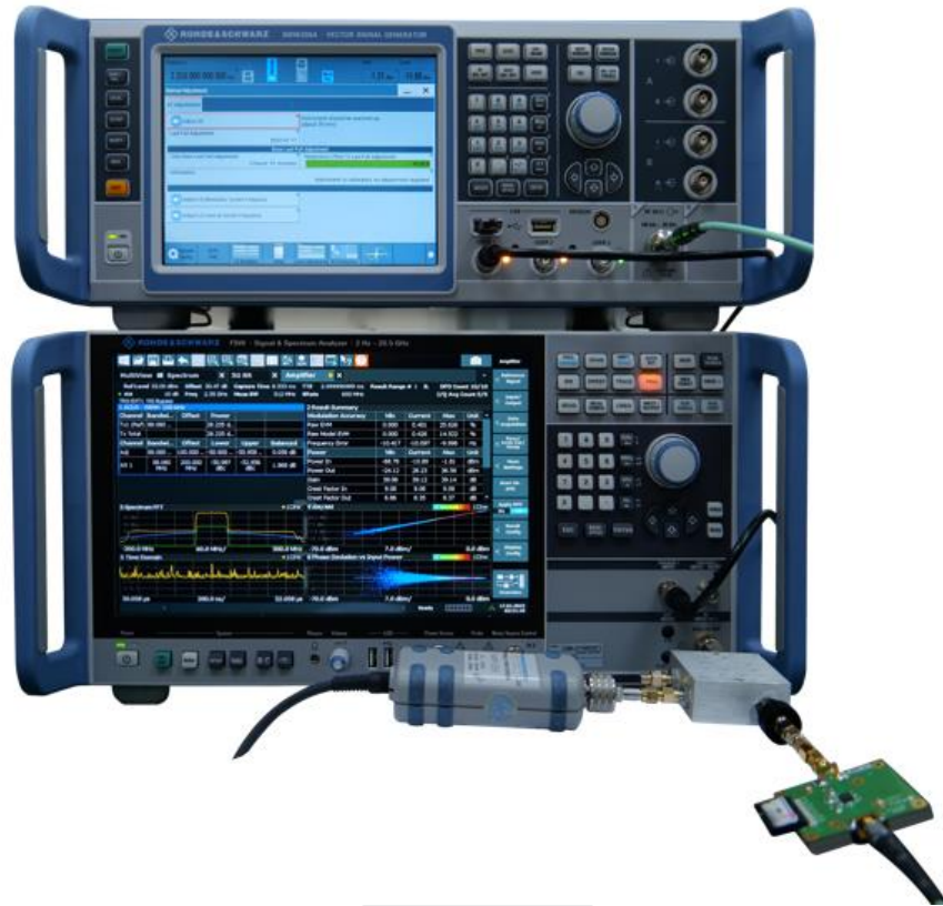
Rohde & Schwarz SMW200A Vector Signal Generator and FSW Signal & Spectrum Analyzer (Photo: arQana Technologies)
