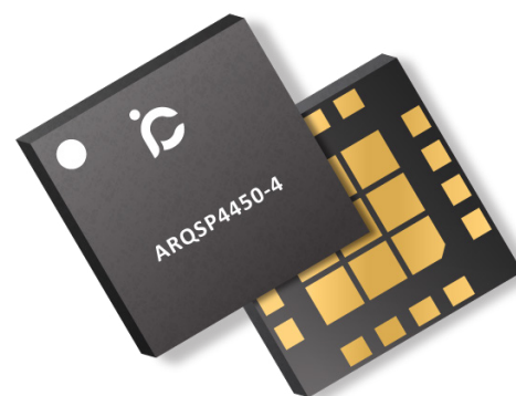
16 Pad 5 \times 5 \text{ mm}^2 LGA Package
